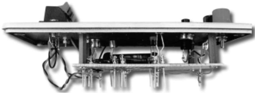
PHOTO 2: Side view of unit with circuit board mounted to cover.
