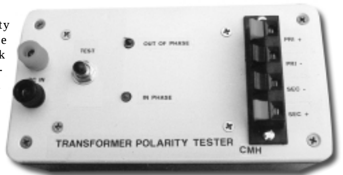
PHOTO 1: The completed polarity tester.
